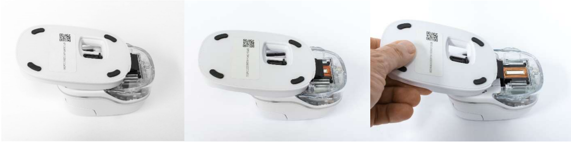
Fig.31: Clean print head with the wiper
